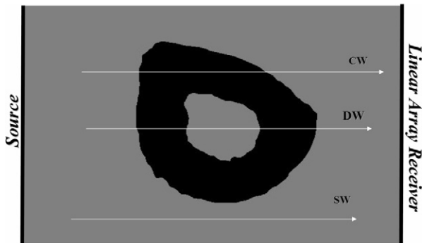
Fig. 2. Schematic of radius bone showing three propagation pathways (see text).
